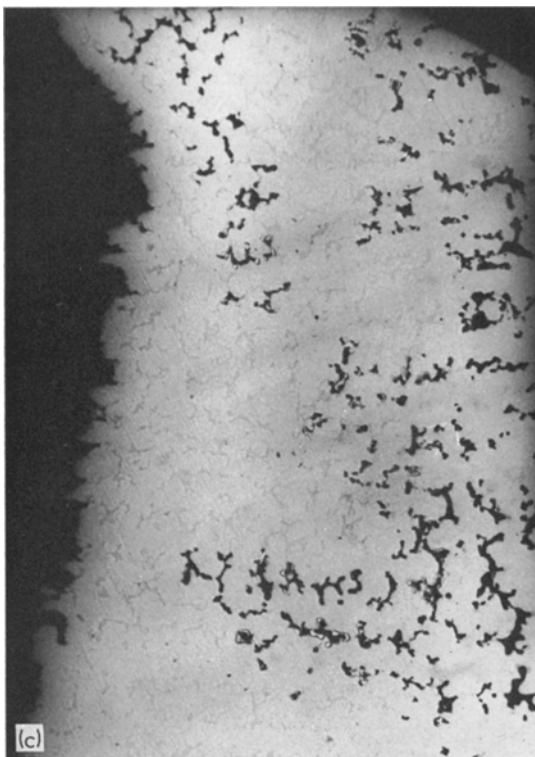
Figure 3 Photographs of a polished section showing the location of porosity near the line of fracture (a) general photograph of the area of study, (b) detail showing the area of porosity (1 mm across) and (c) detail within the area of porosity showing dendritic growth of crystallites. Note: diameter of the bar in (a) is 3 mm.
